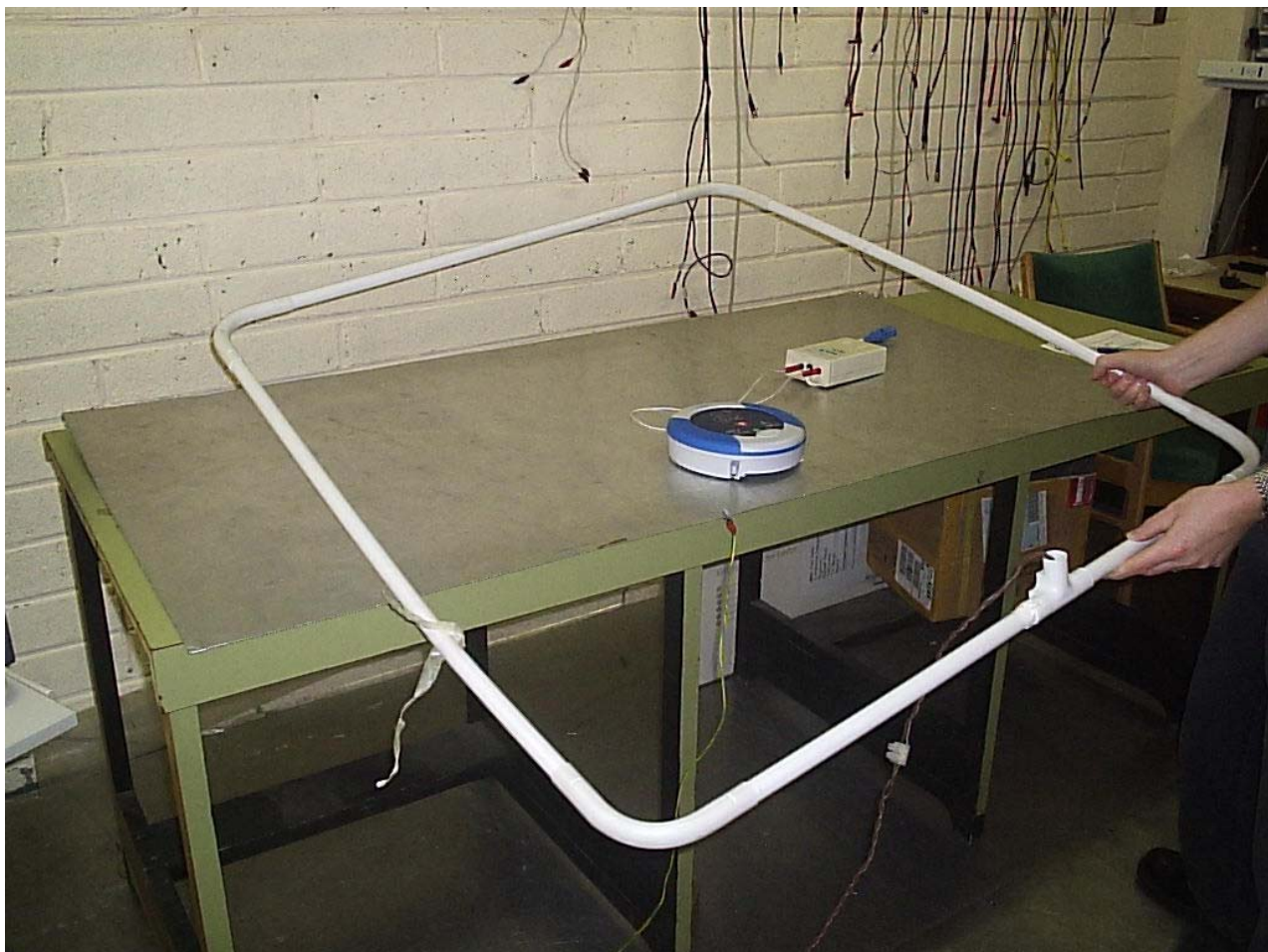
Figure 3: Power frequency magnetic field immunity test
